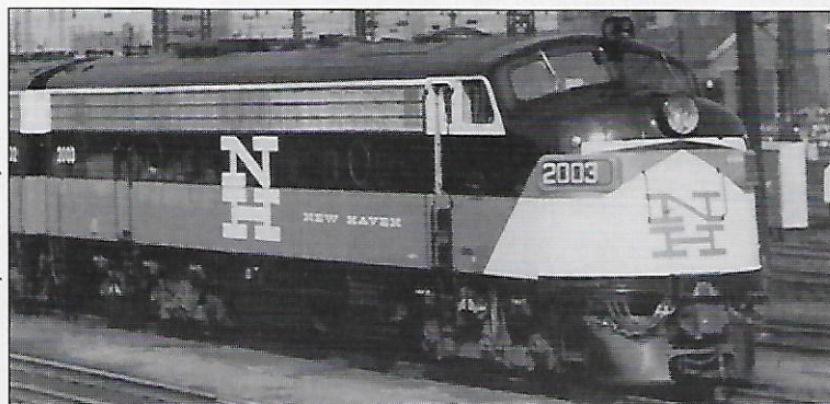
OMI #BA-1111 ▶ NH FL9 "EDER-5a" #2037 [1], 2040 [2], 2055 [3], modified 1960's era w/ safety appliances on RS, 90 degree grab iron above LS windshield, Factory painted red-orange/white/black "McGinnis" scheme, lettered, lights.
